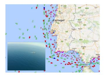
Figure 4-2: Maritime Navigation Corridors off the shore of Mainland Portugal; overlap of the detection and localization of a cargo ship at about 40km from the shore line, obtained from a CIAFA Class-I UAS. Sources: CIAFA and Google Data, 2015.
