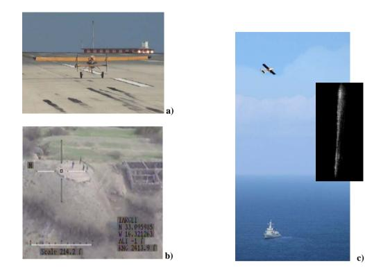
Figure 4-4 – Images of the ZARCO exercise, in Porto Santo. a) take-off of a CIAFA UAS prototype (150kg) from the Porto Santo international airport equipped with electro-optic and Warsaw University's SAR payloads; b) optical image of forces in the field; c) pass over the Navy ship Bartolomeu Dias, and respective radar imagery (radar imagery is copyright from Warsaw University of Technology).
